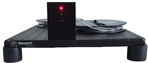
Figure 3. Front view of our artificial binary-star system with the fibers inserted in the L-shape element PS.
