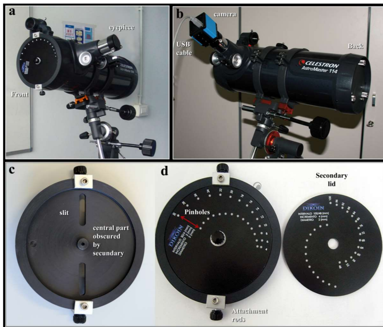
Figure 4. (a) reflector telescope with the lid; (b) telescope with the coupled camera; (c) internal slit; (d) external revolving lids with circular apertures. Separation distances between the pinholes are indicated on the mask in millimeters; the distance is changed by turning the revolving lid.
