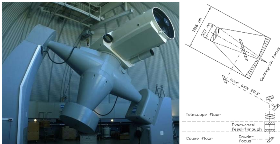
Figure 5 Equatorially mounted 1 m Zeiss telescope of the OGS (left) and Coudé optical path schematics (right)
