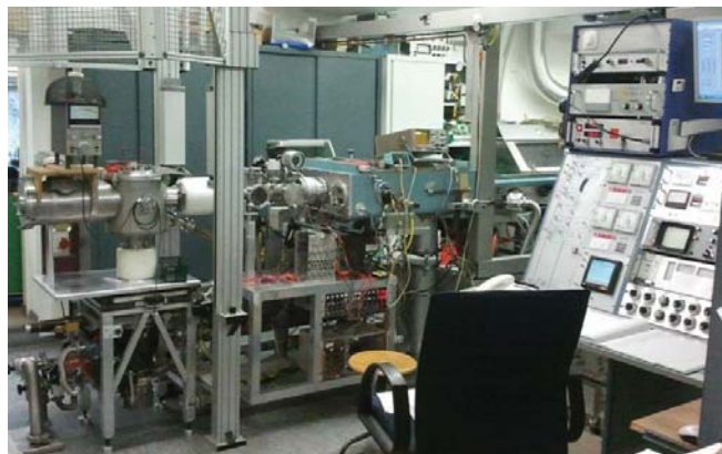
Fig. 1 The isotope separator at the University Bonn used for proton irradiation. The samples were placed in a vacuum chamber.
