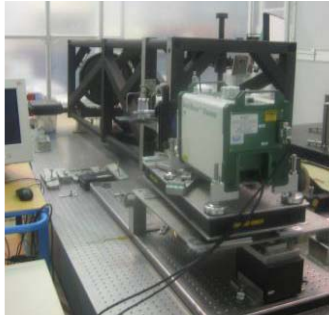
Figure 6. Collimator alignment set-up
