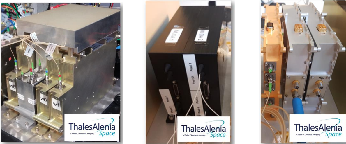
Figure 6. Photonic FGA (left), MLOA (center) and OMC unit (right) of the OWR demonstrator
