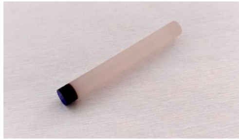
Figure 1. Monolithic, optically bonded Nd:YAG/Cr:YAG laser resonator, 4mm diameter.
