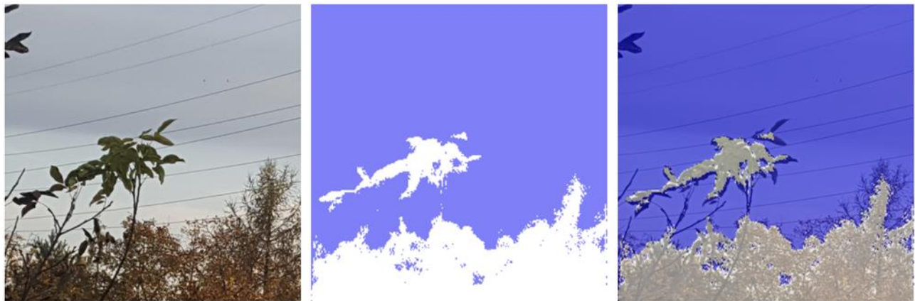
Figure 2. a – input image, b – detected vegetation area, c – comparison of input image and its segmentation.
