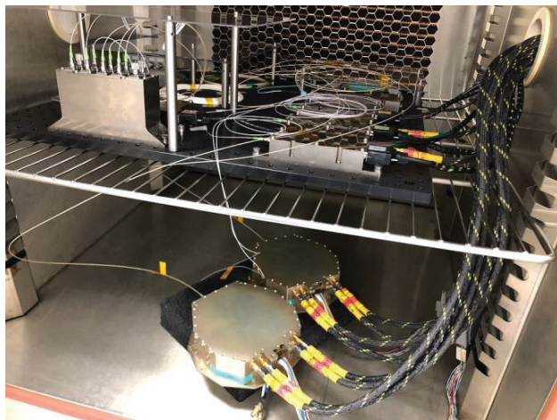
Figure 9. OHA (upper tray) and two ALR receivers (lower tray) inside the climatic chamber for functional testing
