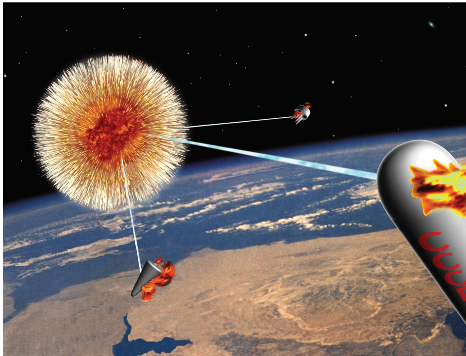
Fig. 1. Conceptual plan for using an X-ray laser for missile defense against the booster, warhead bus, or individual re-entry vehicle (RV) during different phases of an ICBM flight trajectory.
