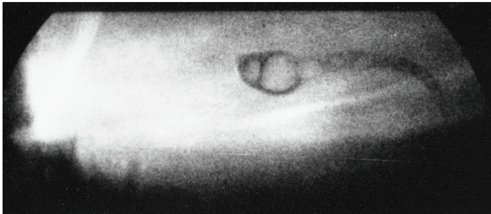
Fig. 5. Image of rat sperm captured using an x-ray microscope that uses the 44.83-nm nickel-like tantalum laser line as the light source. The vertical extent of image is about 10- \mu m. This image shows 50-nm features as described in Ref. 23.
