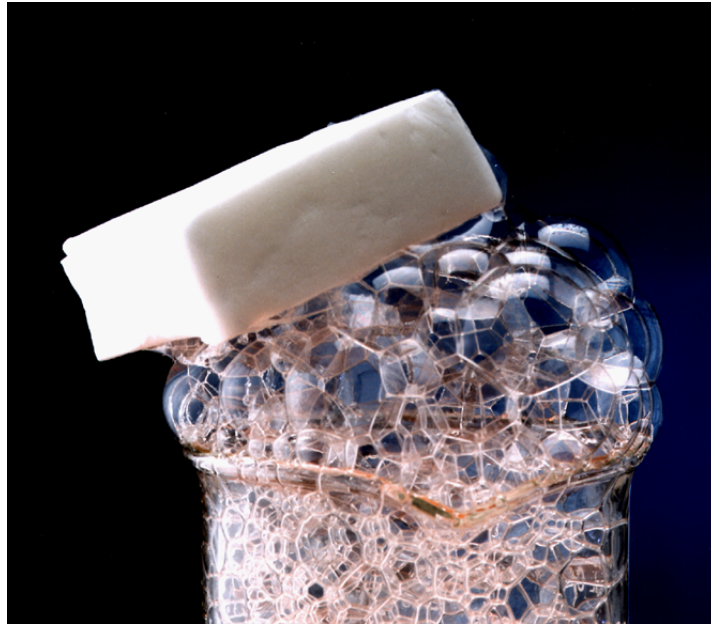
Fig. 4. A piece of SEAgel floating on soap bubbles in a beaker. This very-low-density organic-based foam, made from the food- thickening agent agar, is safe enough to eat and could be used as food packaging or encapsulating material for timed- release medication.
