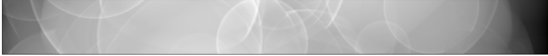
Figure 2. Example projection from the synthetic dataset with different sized water spheres consisting of 80 overlapped detector rows and 800 channels.
