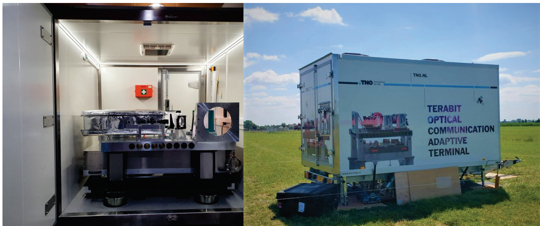
Figure 10: Pictures of TOmCAT BMUX and OGT demonstrators: the full BMUX demonstrator assembled (top); the OGT fully integrated with the BMUX below the main baseplate, covered by aluminium shields (bottom left); complete OGT transported to the test location for the ground-to-ground tests (bottom right).
