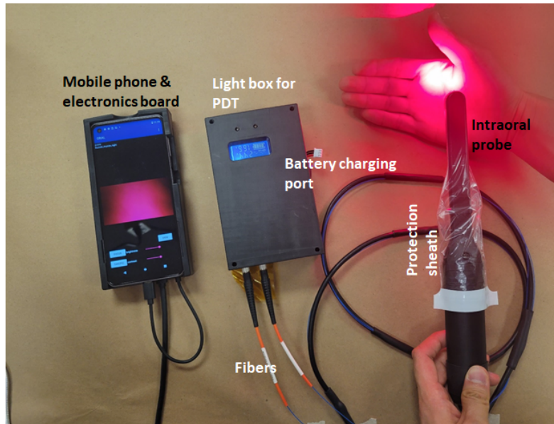
Figure 1. Photos of the intraoral device, electronics board, lightbox, and handheld intraoral probe. The lightbox houses a rechargeable battery, two diode lasers, and a current regulator. This regulator provides data on the driving current and voltage. The battery can be recharged via an integrated USB connector. The handheld probe has an autofocus camera module, which can operate in two distinct imaging modes: autofluorescence and polarized white light.
