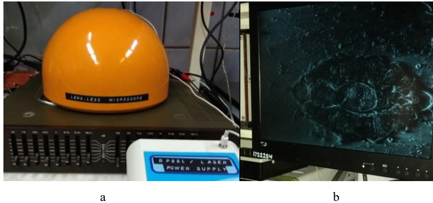
Figure 3. Multispectral holographic lens-less microscope (a) and an example of the resulting analog volume image rendering (3D) of a biosample / histological section for multispectral holographic lens-less microscope with a frequency equalizer (b).
