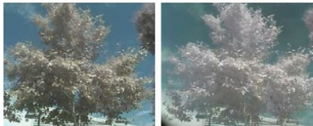
Figure 21. Two images, shown here, of a tree were taken by an OptoBotics Summer Camp student. He used the Rover 2.0 and a linear polarization filter in perpendicular orientations showing the polarization effects.
