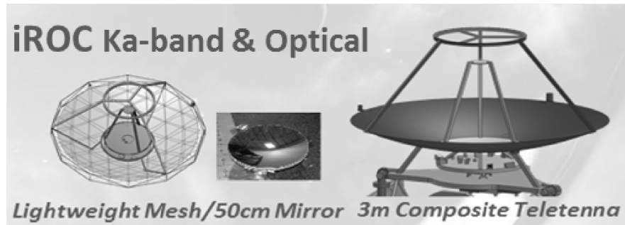
Figure 4. The integrated Radio and Optical Communications (iROC) terminal, a technology investigation to merge Ka-band RF and 1550 nm optical communications within the same size, weight, and power (SWaP) of today's current RF systems. (Figure courtesy of Dr. Daniel Raible, NASA GRC).
