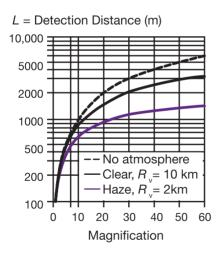
This graph shows the maximum values of L as functions of M and  $R_V$  for three atmospheric conditions when the same target can be detected at 100 m with the unaided eye. Note that a given change in M has less effect on L when the target is at a long distance.
