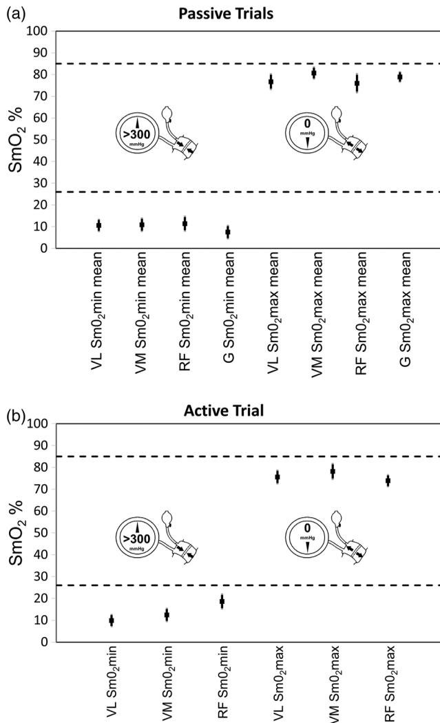
**Fig. 3** Mean (black squares) and 90% CI (thick darker vertical lines) and 95% CI (thin lighter vertical lines) for SmO<sub>2</sub> min and SmO<sub>2</sub> max for (b) active and (a) passive conditions for all muscle sites: VL, VM, RF, and G. Dashed lines indicate the *a priori* determined thresholds of SvO<sub>2</sub> for assessment of face validity.
