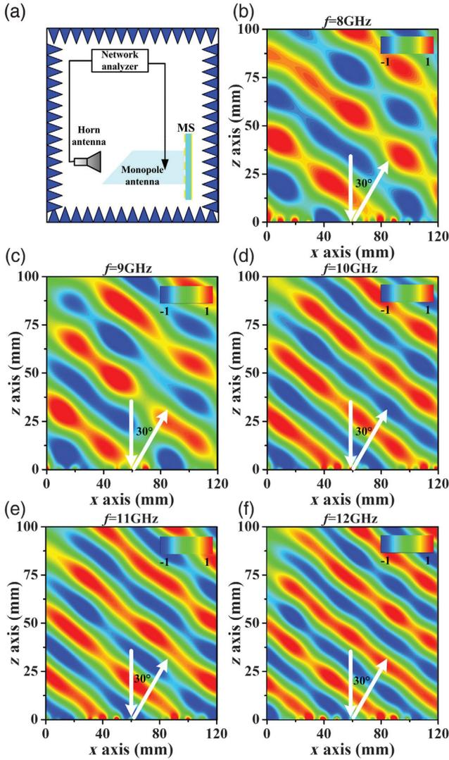
**Fig. 4** Electric field distributions of our meta-device under excitation of  $\hat{x}$ -polarized waves. (a) Experimental setup of the near-field measurement. Measured  $\text{Re}[\vec{E}]$  distributions on the  $xoz$  plane at the reflection side of our metasurface at (b) 8 GHz, (c) 9 GHz, (d) 10 GHz, (e) 11 GHz, and (f) 12 GHz under excitation of normally incident  $\hat{x}$ -polarized waves. All of the electric field spectra are normalized against the maximum value at each frequency.
