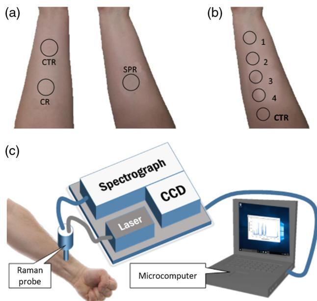
**Fig. 1** (a) and (b) Forearm markings for repellent and sunscreen application in circular sites, respectively. (c) Schematic diagram of the dispersive Raman spectrometer used for spectral data acquisition. The Raman probe possesses a conical aluminum tip to promote the focal distance between the probe tip and the skin surface.
