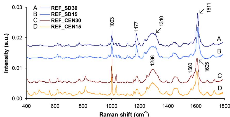
**Fig. 5** Raman spectra of sunscreen products of the two bands CEN and SD in two different SPFs (SPF 15 and 30). The labeled peaks represent the most significative peaks.
