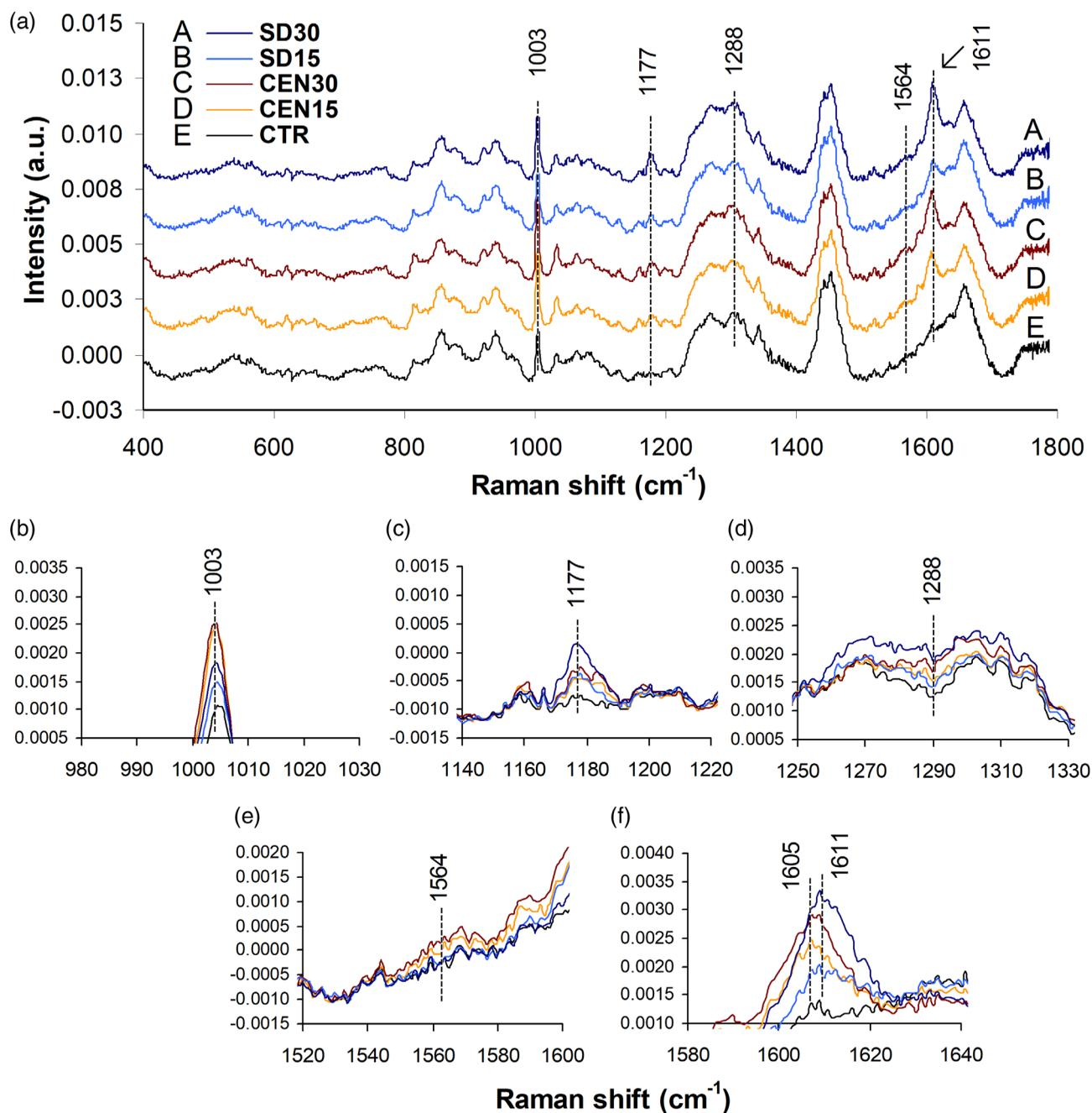
**Fig. 6** (a) Mean Raman spectra of the skin from volunteers with applied sunscreen products (CEN15, CEN30, SD15, and SD30) and from control (CTR). The plots of the peaks at (b) 1003 cm<sup>-1</sup>, (c) 1177 cm<sup>-1</sup>, (d) 1288 cm<sup>-1</sup>, (e) 1564 cm<sup>-1</sup>, and (f) 1605/1611 cm<sup>-1</sup> allow the observation of the overlap of the peaks from CTR, CEN15, CEN30, SD15, and SD30 with the peaks of CTR skin.
