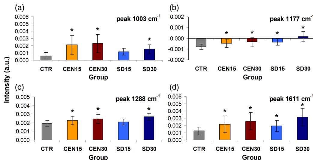
**Fig. 7** Plot of the mean intensity and standard deviation of the Raman peaks of the active ingredients of the sunscreen products found in the spectra of the skin: (a) peak  $1003\text{ cm}^{-1}$ , (b) peak  $1177\text{ cm}^{-1}$ , (c) peak  $1288\text{ cm}^{-1}$ , and (d) peak  $1611\text{ cm}^{-1}$ . The symbol "\*" indicates a statistically significant difference between the groups CEN15, CEN30, SD15, and SD30 versus CTR when indicated ( $p < 0.05$ , ANOVA, and Tukey *post hoc* tests).
