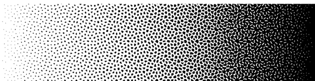
Fig. 9 Gray ramp halftoned with the spot function from Eq. (2) when a_i is varied with H_i and \gamma_i = 1 . This image demonstrates increasing a_i inversely proportionally with H_i .
