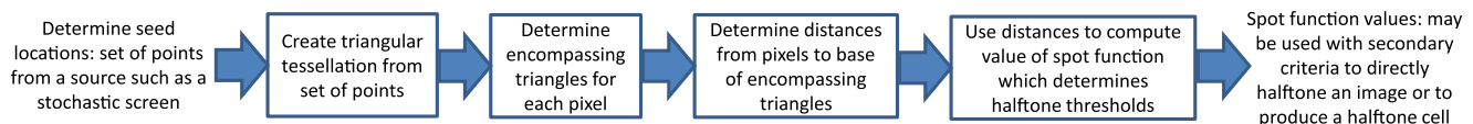
Fig. 1 Schematic illustration of the steps involved in the creation of the halftone spot function values as a function of distances to bases of encompassing triangles.
