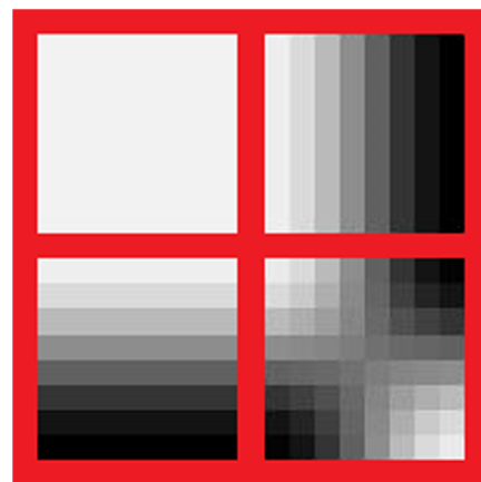
Fig. 16 Graphical representation of first-level DCT basis functions.
