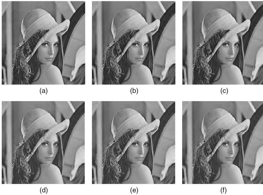
Fig. 5 Lena images obtained at a bit rate of 0.1 bpp: (a) original image, (b) SPIHT peak signal-to-noise ratio (PSNR) = 29.81 dB, (c) modified SPIHT PSNR = 29.82 dB, (d) set partitioning in hierarchical frequency bands (SPHFB) PSNR = 30.31 dB, (e) LMSPIHT PSNR = 31.21 dB, and (f) Fang et al. PSNR = 29.81 dB.
