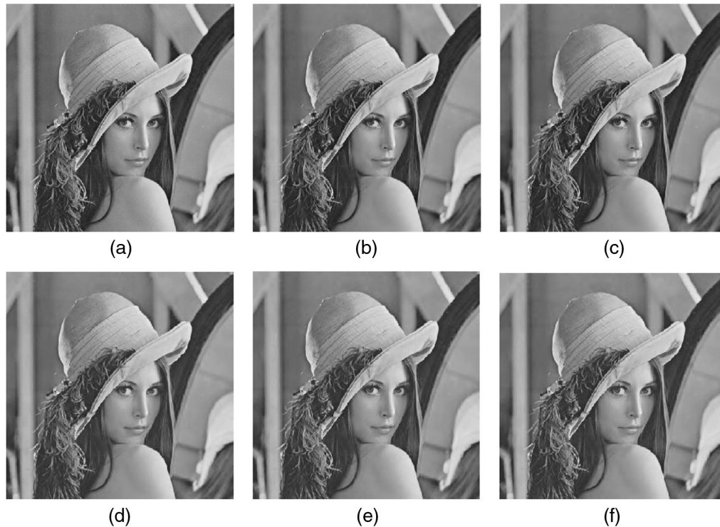
Fig. 7 Lena images obtained at a bit rate of 0.5 bpp: (a) original image, (b) SPIHT PSNR = 36.78 dB, (c) modified SPIHT PSNR = 36.78 dB, (d) SPHFB PSNR = 36.78 dB, (e) LMSPIHT PSNR = 36.80 dB, and (f) Fang et al. PSNR = 36.78 dB.
