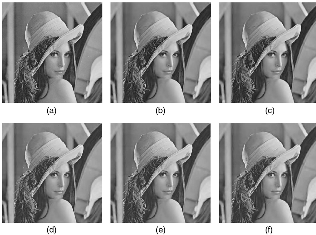
Fig. 6 Lena images obtained at a bit rate of 0.25 bpp: (a) original image, (b) SPIHT PSNR = 33.65 dB, (c) modified SPIHT PSNR = 33.65 dB, (d) SPHFB PSNR = 34.15 dB, (e) LMSPIHT PSNR = 34.88 dB, and (f) Fang et al. PSNR = 33.65 dB.
