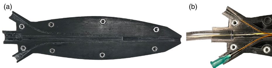
Fig. 8 (a) Open handle showing the internal channels guiding the different components and (b) handle with components installed.
