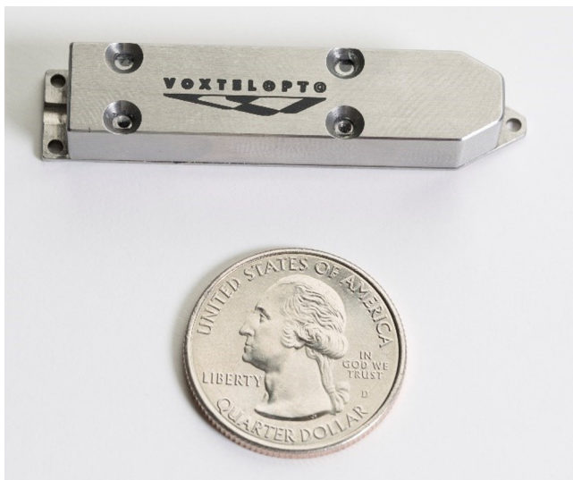
Fig. 5 Picture of Voxtel's miniature 1535-nm DPSS laser, which has a beam quality of M^2 < 1.1 * \text{DL} (diffraction limit) and operates at 20 \mu\text{J} at up to 400-kHz repetition rates.
