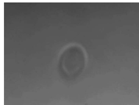
Video 1. A single RBC can be repeatedly stretched using a 1 \times 3 \mu\text{m} optical stretcher (1.9 MB). [URL: http://dx.doi.org/10.1117/1.3470124.1 ].
