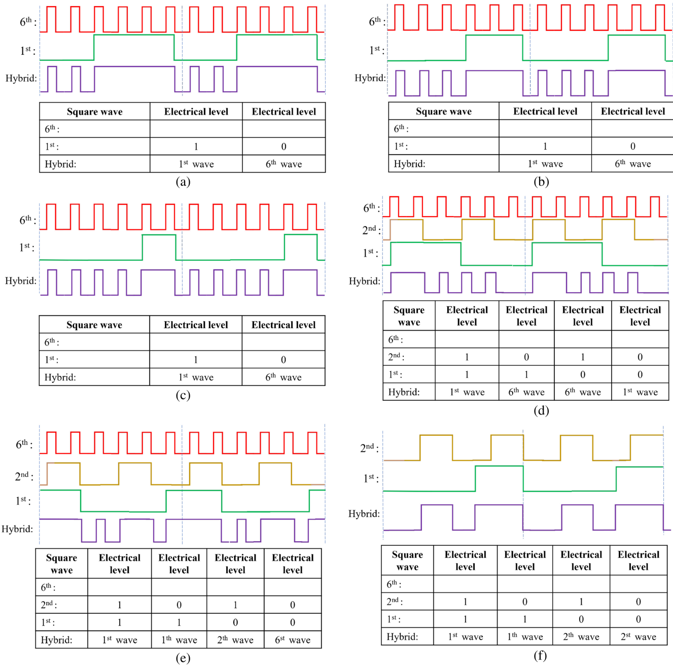
Fig. 10 The composition analysis of the nonuniform square waves measured in Fig. 9. (a) Fig. 9(a-i), (b) Fig. 9(b-i), (c) Fig. 9(c-i), (d) Fig. 9(d-i), (e) Fig. 9(e-i), and (f) Fig. 9(f-i).
