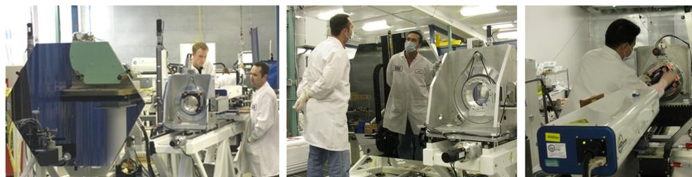
**Fig. 7** OTS CoC interferometric CGH null test simultaneously measures conic constant, radius of curvature, prescription alignment, and surface figure error. Pallet contains 4D PhaseCAM, diffraction international CGH on a rotation mount, and Leica ADM. PMSA mount rotates for six position tests. Quad cell alignment aids attach to PMSA.
