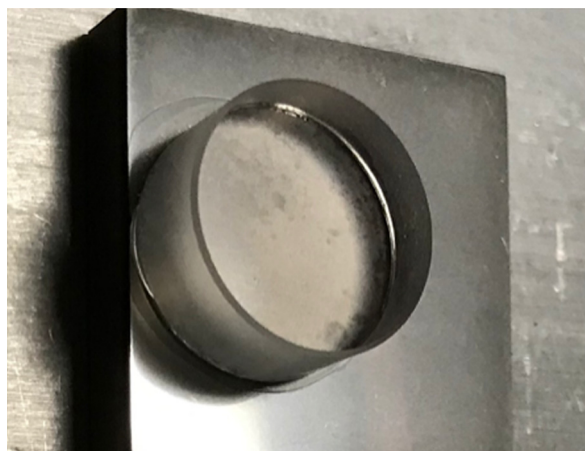
Fig. 1 Allvar–glass HCB bond, which exhibits visible transparency.
