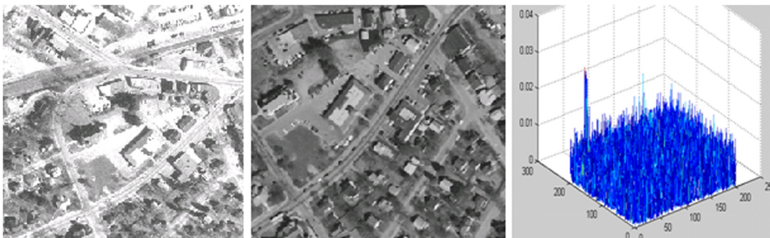
Fig. 7 Utilize Fourier–Mellin transform (FMT) to roughly estimate the rotation angle of the two images.
