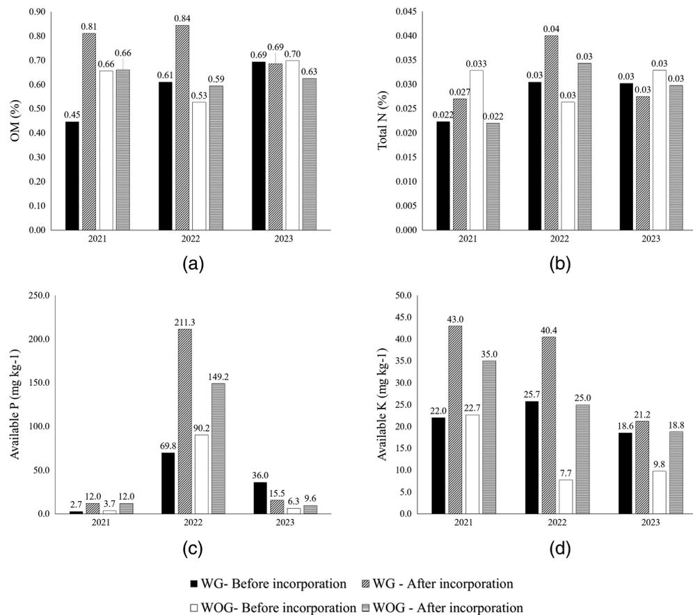
**Fig. 3** Changes in key soil properties in the experimental plots during 2021 to 2023. (a) Soil OM (%), (b) total nitrogen (%), (c) available phosphorus (mg/kg), and (d) available potassium (mg/kg) were measured in the green manure-amended plots (WG) and control plots WOG before and after incorporation.
