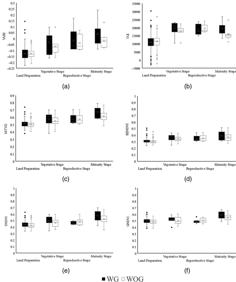
**Fig. 5** VIs at the vegetative stage of rice with *C. ensiformis* green manure (WG) and soil without green manure (WOG). These VIs included VARI (a), TGI (b), MTVI2 (c), RENDVI (d), YNDVI (e), and GNDVI (f).
