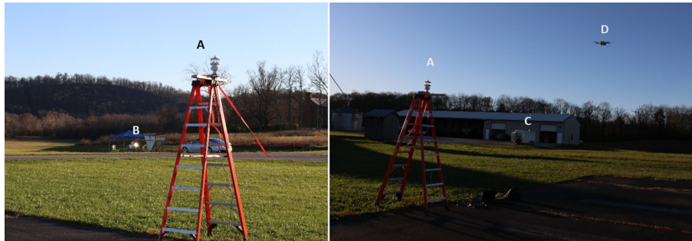
Fig. 3 Pictures taken near reference position. The sonic anemometer marked “A” is in the foreground at the reference position. Lidar 1 on the image on the left is marked “B,” and lidar 2 in the image on the right is marked by “C”. Above lidar 2 in the image on the right is the UVA-operated sUAS marked by “D.”
