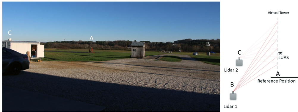
Fig. 11 Image and Illustration of KEAS Virtual Tower experimental setup where “A” is the reference position, “B” is Lidar 1, and “C” is Lidar 2.
