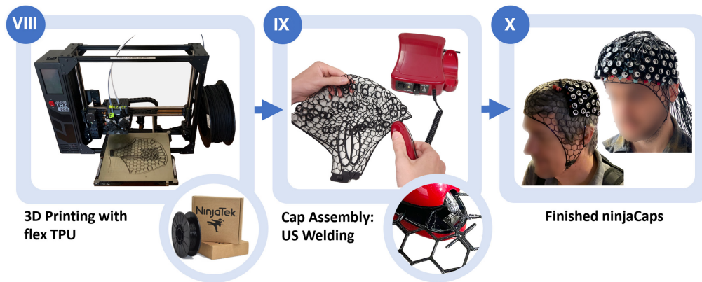
Fig. 8 (VIII) 3D printing of four cap panels. (IX) Manual assembly using ultrasonic welding clamp. (X) Finished ninjaCaps.
