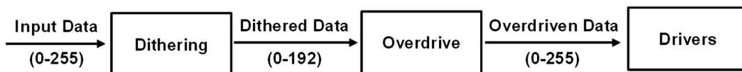
Fig. 6 Schematic diagram of the proposed driving technology for improving motion quality of AMOLED.
