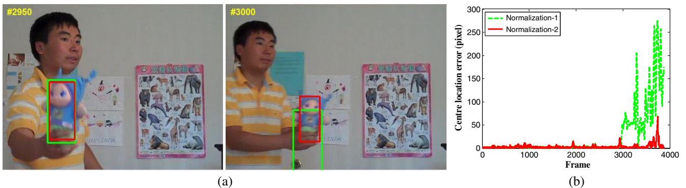
Fig. 4 Comparisons for two trackers based on different normalizations (red bounding box and line represent 32 \times 16 normalization while green ones represent 32 \times 32 normalization). (a) The tracking results of two trackers based on different normalizations and (b) CLEs of two trackers based on different normalizations.
