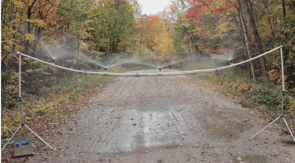
**Fig. 28** A simple rainfall simulator commonly implemented in the film industry (Tom Antos Film).
