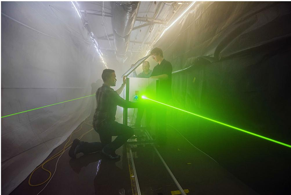
**Fig. 27** The fog facility at Sandia National Laboratory, using lasers to measure and calibrate transmission.<sup>23</sup>
