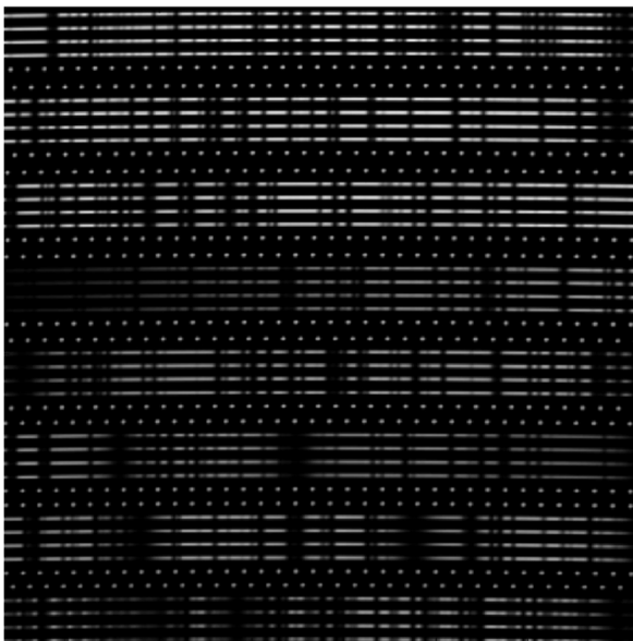
Fig. 7 A subsection of a simulated MINERVA echellogram showing four science spectra bracketed by a simulated stabilized etalon wavelength source. Each science fiber trace represents the input from one of the four MINERVA telescopes that will be observing the same astronomical target.
