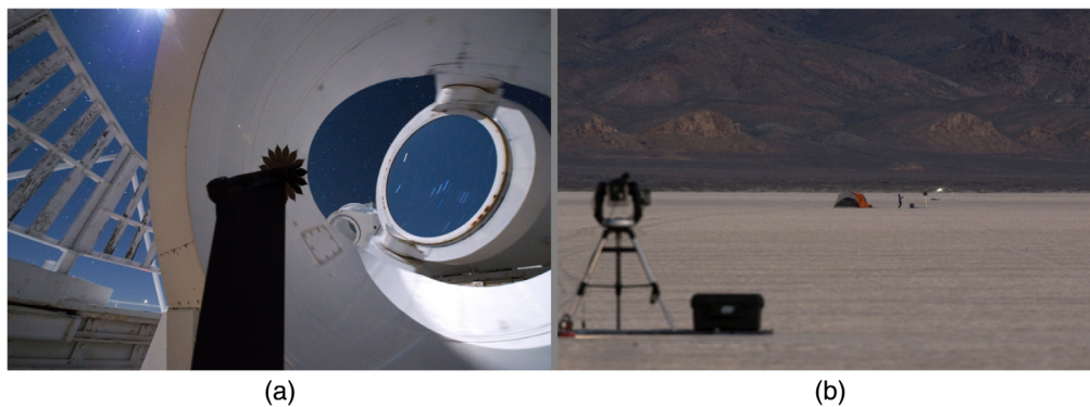
Fig. 8 (a) A starshade is used to observe stars with the heliostat at the McMath-Pierce Solar Telescope. 37,38 (b) A starshade is tested over kilometers of separation on a dry lake bed. 34–36 Photo credit: Robert Brown (Northrop Grumman).
