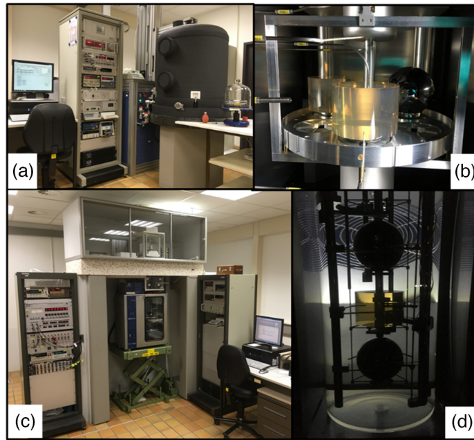
Fig. 3 (a) The cloche protecting the mass comparator from thermal noise and convective flow. (b) ZERODUR® coupon in the weighing basket. (c) Overview of the hydrostatic weighing scale. (d) Closer view of the hydrostatic scale with a ZERODUR® coupon located in the middle basket - below and above Si density standard used for determining the actual density of the immersion fluid.
