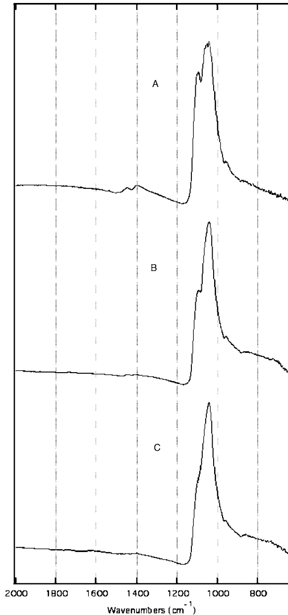
Fig. 6 Spectra by FTIR microscopy were acquired from the different regions of the remineralized 3 day lesion. (a) Sound enamel spectra with the characteristic peaks due to the phosphate group in carbonated hydroxyapatite near 1000\text{ cm}^{-1} and the two smaller peaks near 1400\text{ cm}^{-1} due to the carbonate group. (b) Spectra of the lesion body shows that the carbonate group is absent, which is likely due to the preferential loss of carbonate during demineralization. (c) The outer remineralization layer displays narrow characteristic hydroxyapatite bands, indicating high crystallinity, with an absence of the higher solubility carbonate substitution group.
