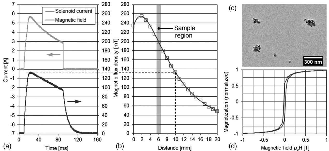
**Fig. 1** Pulsed magnetic field and magnetic nanoparticles: (a) Current pulse using a capacitor charging voltage of 120 V and resulting magnetic flux density measured 10 mm above the solenoid's surface. (b) Peak magnetic flux density versus axial distance from solenoid. (c) Electron microscopy image and (d) magnetization curve of the applied magnetic nanoparticles.
