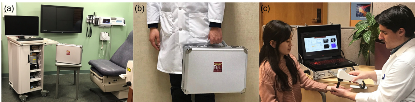
Fig. 3 Portability of the briefcase OCT system. (a) Comparison of the briefcase OCT system with a high-end, cart-based LCI system. (b–c) Photographs illustrating the portability of briefcase OCT where a physician can easily carry such system for examination in primary care and point-of-care settings.
