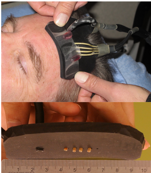
Fig. 1 NIRS probe used in this study. Unlike conventional probes, this probe is not flushed with fiber but has protruding fibers instead. This allows measurement in regions with hair, by combing the hair apart and exposing the scalp.
