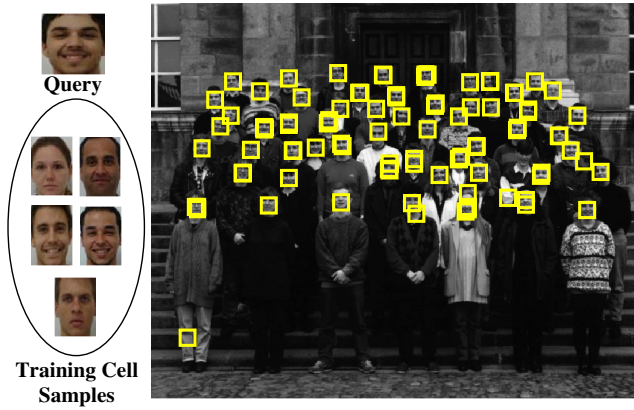
Fig. 9 There are 57 faces in the target image, and our method detects 56 faces with five false alarm. \tau_L = 0.7812 , \tau_S = 0.7793 , \tau_\theta = 0.7704 , and \tau_h = 475.1 .
