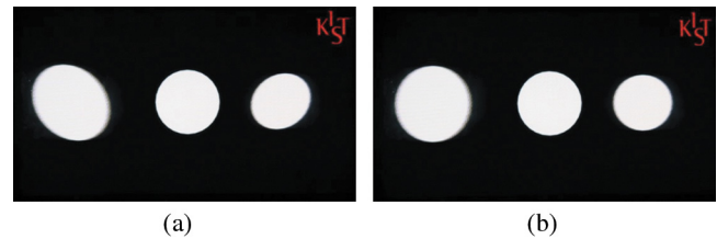
Fig. 9 Example of correction of 3-D image in a misaligned 3-D display: the left one has -220 mm depth, the center one has no depth, and the right one has +220 mm depth. (a) Before correction and (b) after correction by skewing 3-D objects.
