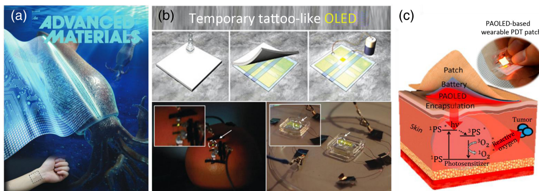
Fig. 3 (a) Schematic illustration of chitin nanofiber transparent paper for flexible green electronics. Adapted with permission from Ref. 63, ©2016 Wiley-VCH Verlag GmbH & Co. KGaA, Weinheim. (b) Transfer process of the OLED tattoo device and picture presenting working OLED tattoo transferred on an organic as well as a PVF nanosheet. Reproduced and adapted with permission from Ref. 64, ©2021 Wiley-VCH Verlag GmbH & Co. KGaA. (c) Schematic illustration of the photodynamic therapy (PDT) treatment principle and a photo of the wearable OLED-based PDT patch. Reproduced and adapted with permission from Ref. 65, ©2020 American Chemical Society.
