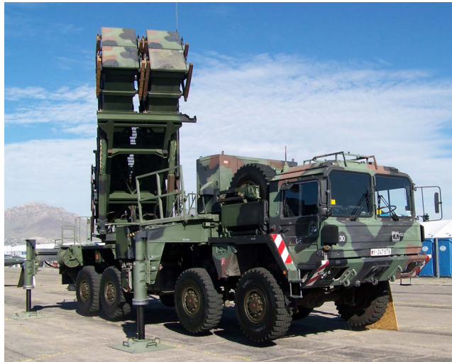
Fig. 2 Transporter-erector-launcher (TEL) vehicle for U.S. Patriot SAM system with four rectangular missile launch canisters. The TEL is shown in the erect position ready for missile launch.
