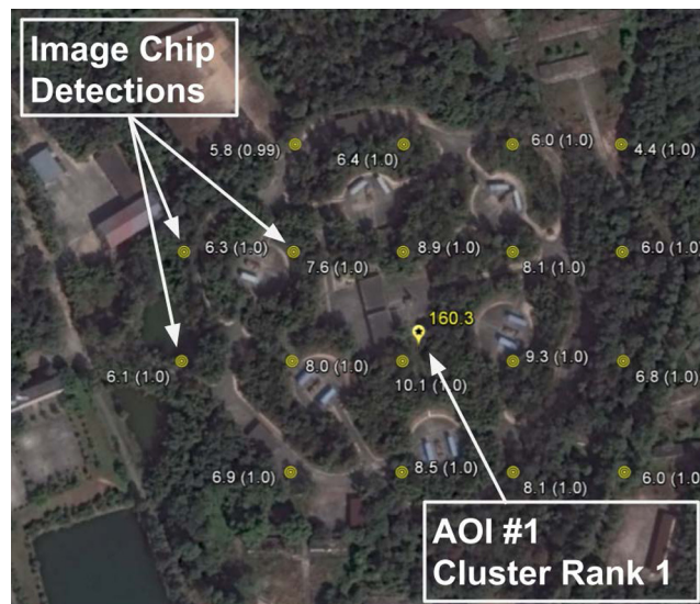
Fig. 12 DCNN detection density surface generated for a candidate SAM site in Aol 1. The image chip centers (bullseyes) are labeled with the spatially amplified density value followed by the DCNN output confidence in parentheses. The cluster center (yellow placemark) is measured as the sum of the densities (160.3) that aggregate into this cluster's overall score. The overall cluster score is then used to rank order (high to low) the candidate SAM sites for subsequent human review.
