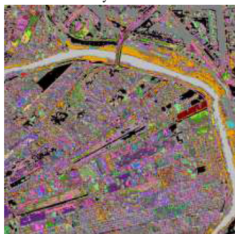
Fig. 6 Partitioning the hyperspectral image of Fig. 2(a) based on the parameter p .
