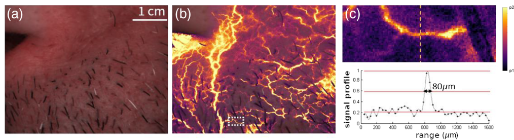
Fig. 4 Evaluation of the spatial resolution of the LSOCl instrument. (a) Example of color image near the nose for which we overlay the microvascular activity image in (b). (c) A cross section analysis of a fine vessel squared in (b) exhibits a full width at half maximum of 80 \mu\text{m} .
