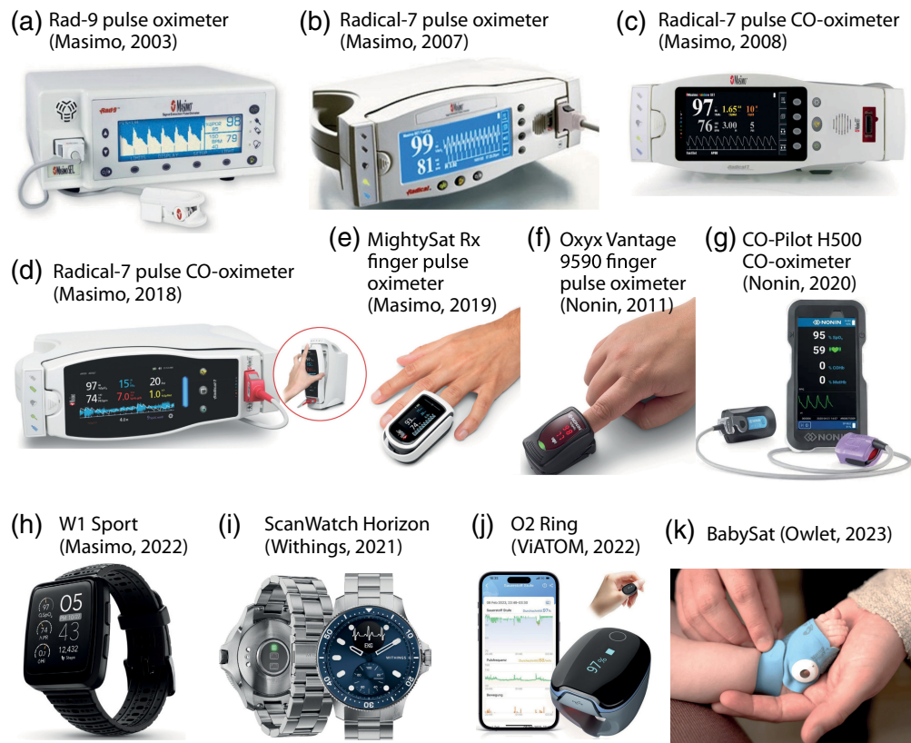
Fig. 8 Examples of POs and pulse CO-oximeters developed in the 2000s, 2010s, and 2020s. (a) Rad-9 PO (Masimo). (b) Radical-7 PO. (c), (d) Two versions of the Radical-7 pulse CO-oximeter with the rainbow SET technology. (e) MightySatRx finger PO (Masimo). Images (a)–(e) from the Masimo website. (f) Oxyx Vantage 9590 finger PO (Nonin). (g) CO-Pilot H500 pulse CO-oximeter (Nonin). Images (f) and (g) from the Nonin website. (h) W1 Sport PO smart watch (Masimo). Image from the Masimo website. (i) Scan Watch Horizon PO smart watch (Withings). Image from the Withings website. (j) O 2 Ring (ViATOM). Image from the ViATOM website. (k) BabySat (Owlet). Image from the Owlet website.
