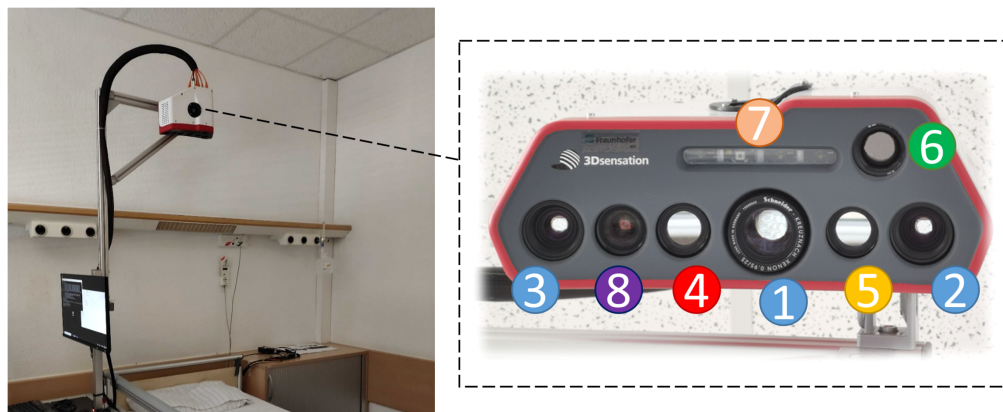
Fig. 6 Multimodal camera system with sensor head composed of a GOBO projector (1), two NIR cameras at 850 nm (2, 3), NIR camera at 780 nm (4), NIR camera at 940 nm (5), thermal camera (6), LED array with LEDs at 780 and 940 nm (7), and color camera (8).
