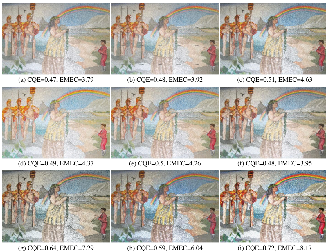
Fig. 10 Experimental results on an overexposure image. (a) Original color image, and others are the results of (b) MSRRCR, 10,38 (c) RACE, 12 (d) Ref. 20, (e) Ref. 24, (f) Ref. 25, (g) Ref. 35, (h) Ref. 23, and (i) the proposed approach.
