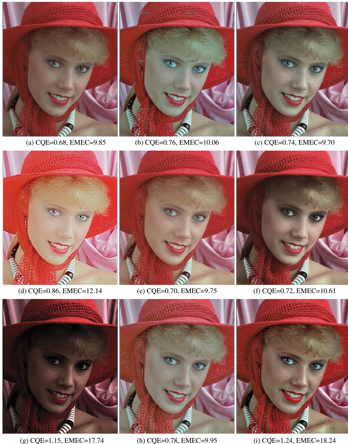
Fig. 17 Experimental results on an image with normal exposure. (a) Original color image, and others are the results of (b) MSRCR, 10,38 (c) RACE, 12 (d) Ref. 20, (e) Ref. 24, (f) Ref. 25, (g) Ref. 35, (h) Ref. 23, and (i) the proposed approach.
